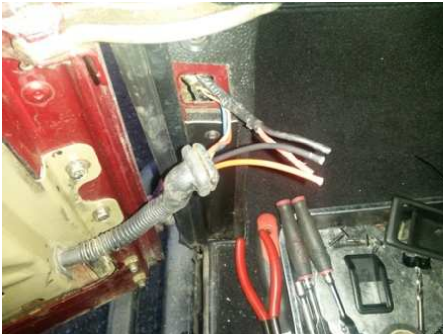
Step 13. I routed my cables from the doors through the rubber conduit to the bulk head where my electric windows and central door locking plugs are. I made the connections via a two way waterproof connector. "Sorry but missed that photo! Must have been getting excited" (See picture below)
