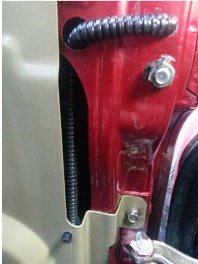
Step 12. Making sure the convoluted tube is sealed. I used Dum Dum sealer the same as Land Rover use on the door plastic membrane. (See picture below)
