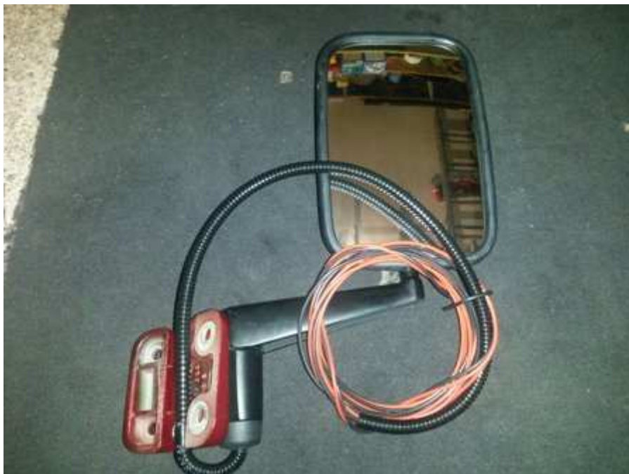
"In the picture above I secured the convoluted tube to the Hinge back via a plastic Black Nylon 'P' Clip secured via the excising mirror arm screw"
