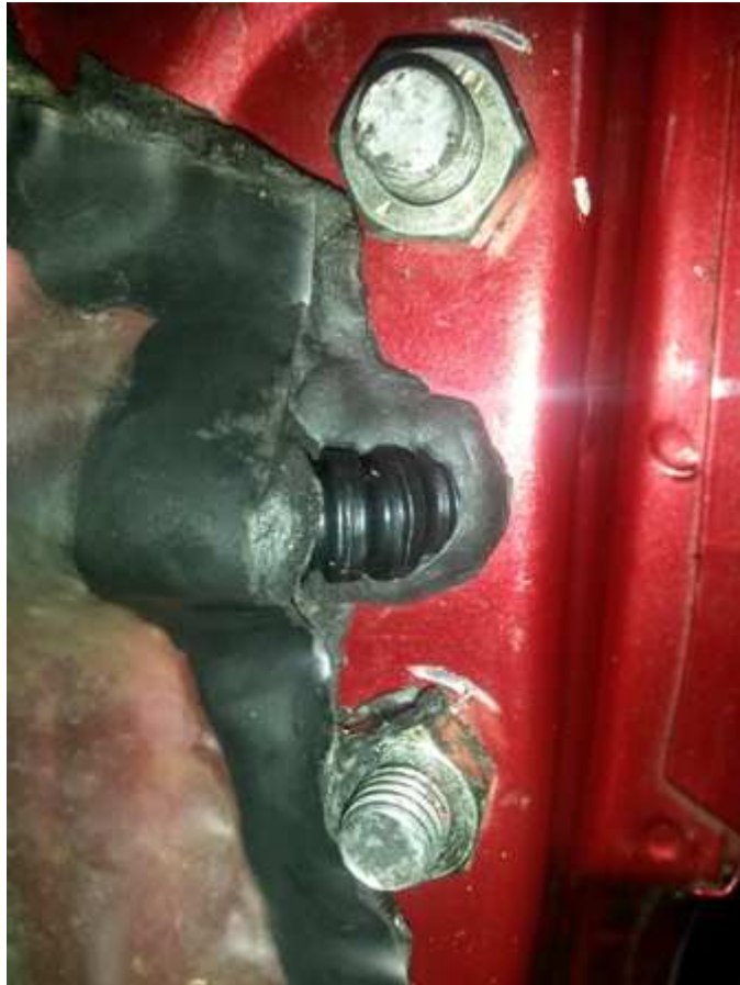
Step 13. I routed my cables from the doors through the rubber conduit to the bulk head where my electric windows and central door locking plugs are. I made the connections via a two way waterproof connector. "Sorry but missed that photo! Must have been getting excited" (See picture below)
