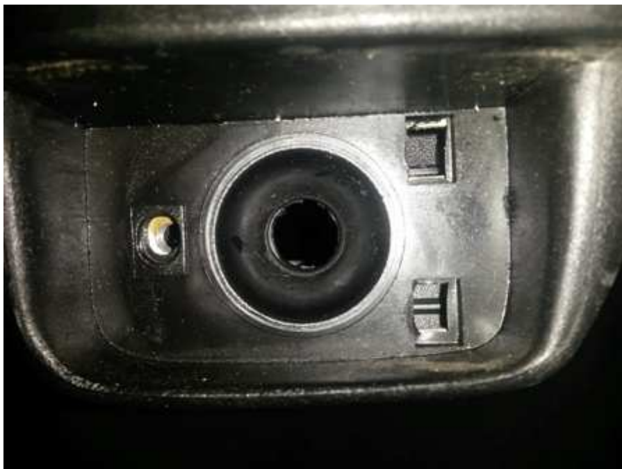
Step 3. I next drilled a hole through the bottom of my mirror casings and through the inside plastic retaining plate, this plate pull slides out (See pictures below)
