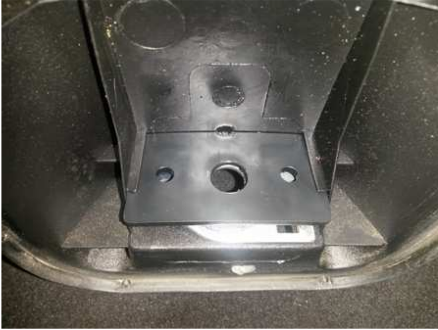
Step 4. I drilled an 8mm hole through the ball end of the arm (See picture below)
