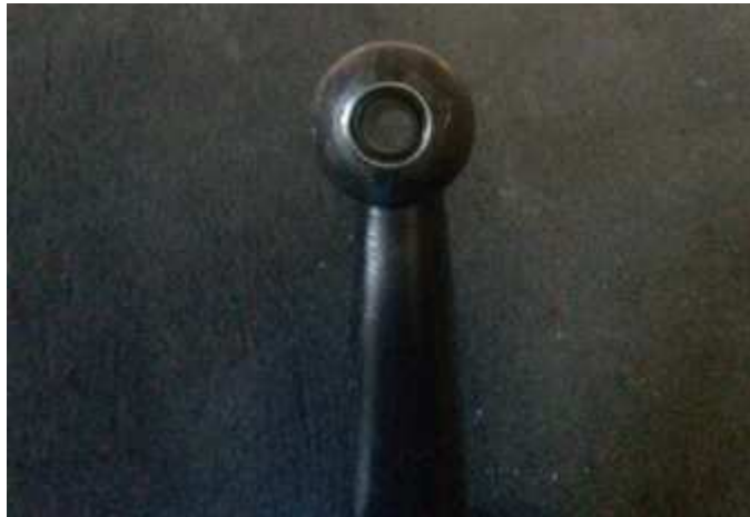
Step 4. I drilled an 8mm hole through the ball end of the arm (See picture below)
